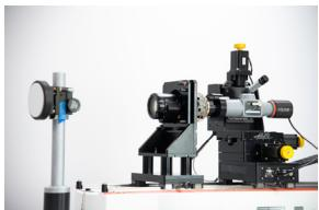
In addition to opto-mechanical design and manufacturing, Optikos services include IQ Lab™ testing by expert optical engineers to ensure that each lens meets specifications and, if needed, we are able to incorporate the imager into the assembly to ensure proper focus and imager alignment and verified performance.
