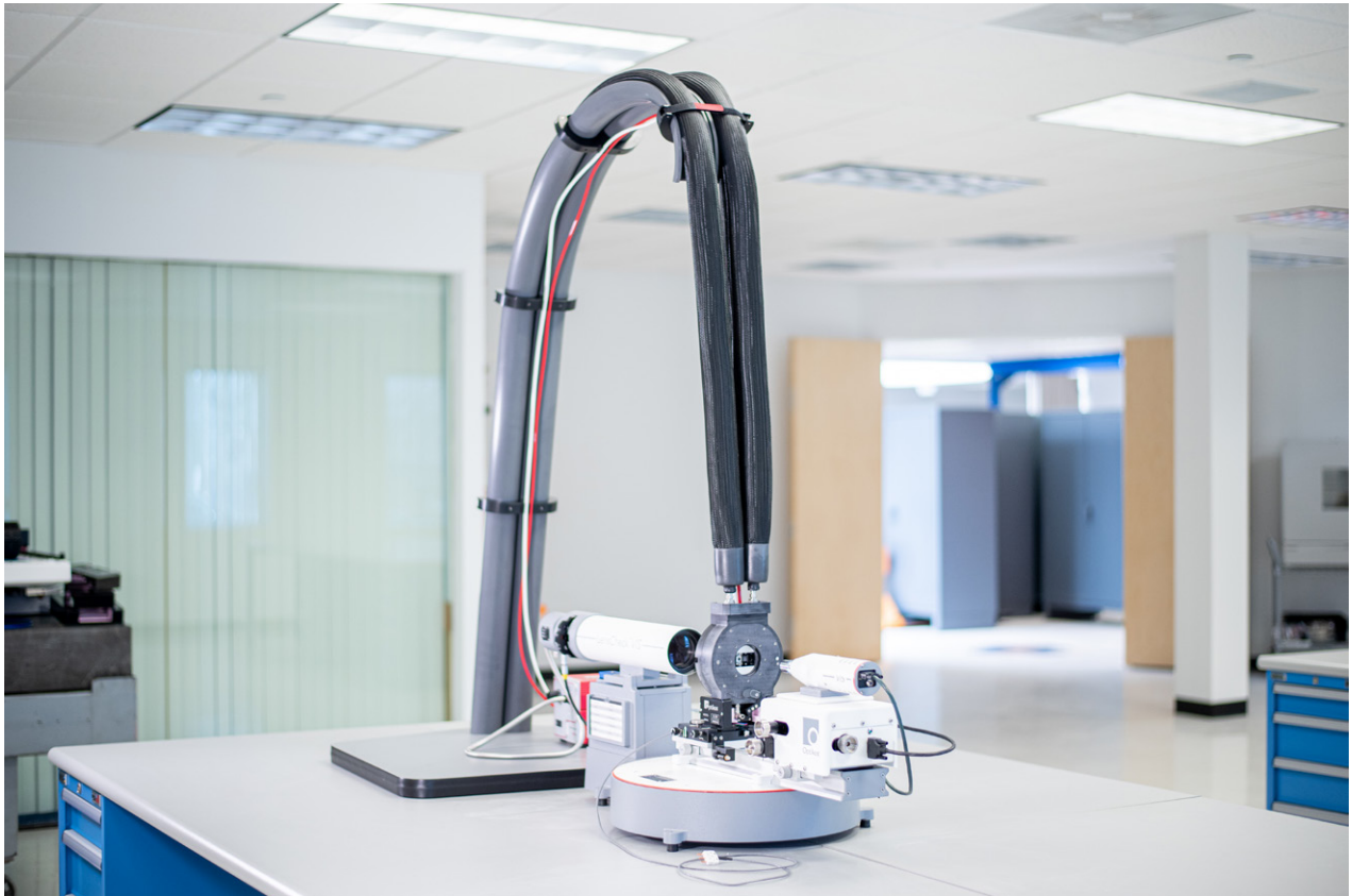
LensCheck VIS with Thermal Chamber and Sky Hook (Temperature Controller and Manifold not shown)
