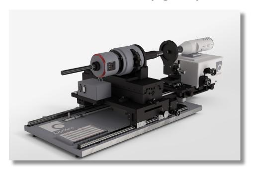
The LensCheck Small Format Finite Conjugate System is configured for measuring MTF and other properties of lenses designed for close conjugate imaging. This compact system allows measurements at object distances from 0 to 300mm, over field diagonals up to 250 mm. It's available as a stand-alone system, or as an accessory to the standard LensCheck VIS system used for infinite conjugate measurements.
