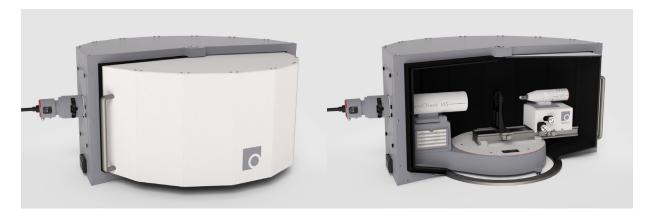
LensCheck™ VIS measurement accuracy and repeatability is optimized when the system is operating in a dark environment that eliminates all stray background illumination. This is especially critical for high dynamic range measurements such as the Glare Spread Function (GSF). The LensCheck Enclosure was designed for this purpose as it replaces the need to provide a dedicated dark room for lens testing.
