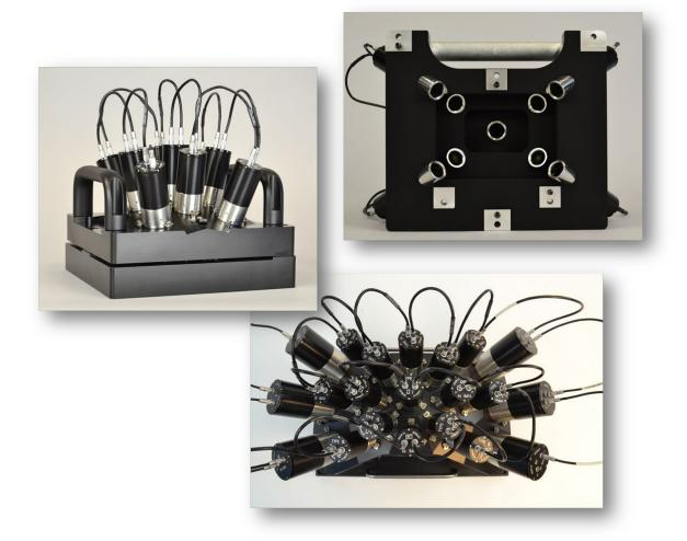
The Meridian Starfield mount consists of a thick plate into which precision bores are machined to receive the target projector barrels. This allows for consistent and repeatable testing of field points. When provided with a customer's camera lens prescription or black box model, Optikos can design unique targets to compensate for high distortion field points for ultra wide FOV cameras.
