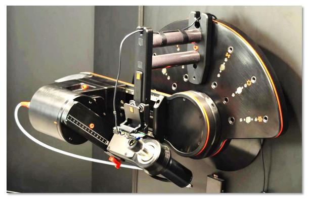
Meridian FLEX with the FieldPoint application will measure multiple optical parameters of cameras, including:
