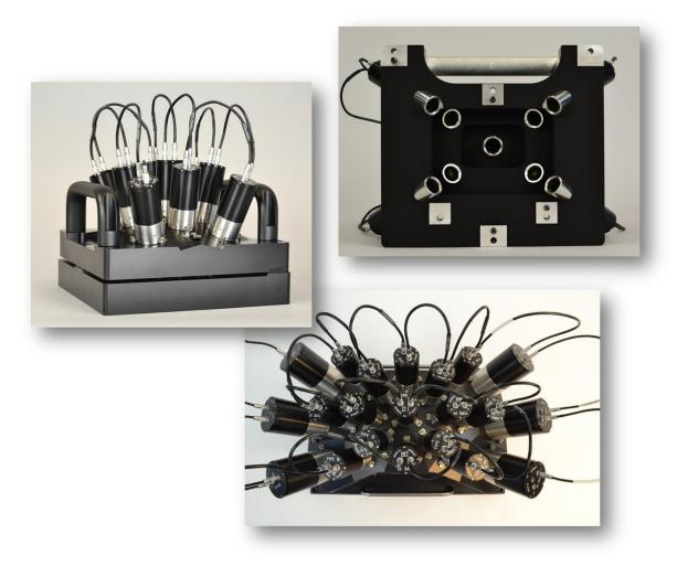
The Meridian Starfield mount consists of a thick plate into which precision bores are machined to receive the target projector barrels. This allows for consistent and repeatable testing of field points. When provided with a customer's camera lens prescription or black box model, Optikos can design unique targets to compensate for high distortion field points for ultra wide FOV cameras.
