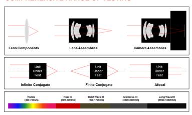
Image quality testing is offered for lenses, cameras, optical and electro-optical components and systems; measurements can be performed for test spectrums ranging from visible to Long Wave Infrared (LWIR), and for infinite conjugate, finite conjugate and afocal To complement our image systems. quality metrology capabilities, additional measurements offered by Optikos IQ Lab Services include radiometric photometric characterization, optical element inspection, and interferometric testing.
