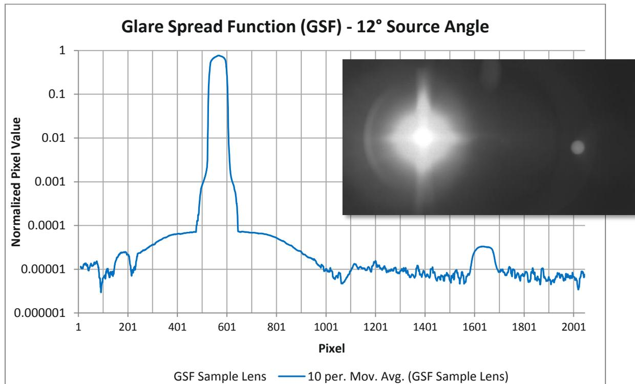
**Figure 6 - Horizontal GSF with a lens 12° off-axis. The dynamic range is greater than  $10^6$ . The inset image shows a very long exposure image. Five images with varying exposure times were combined to create the GSF plot.**
