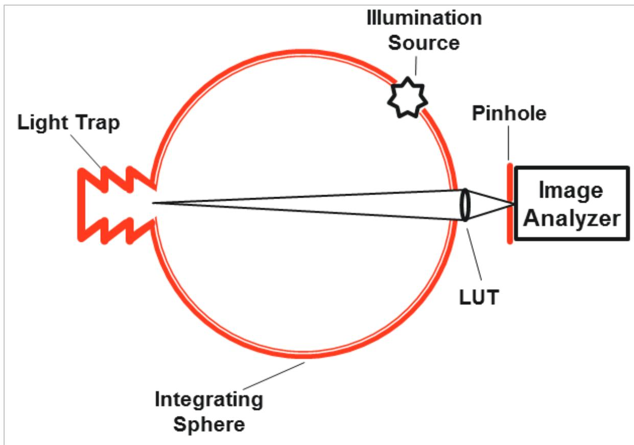
Figure 1 - Instrumentation schematic. The Lens Under Test (LUT) is placed at the entrance port of the integrating sphere.
