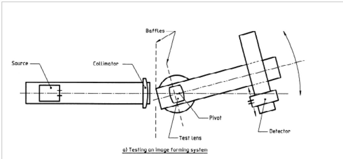
Figure 4 – ISO 9598 Illustration of GSF Measurement
