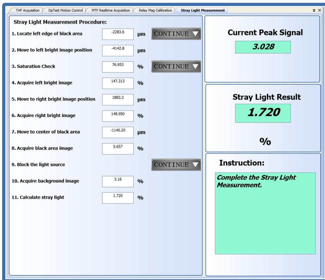
**Figure 3 - The OpTest<sup>®</sup> 7 Interface for Performing Veiling Glare Index (Stray Light) Measurements**
