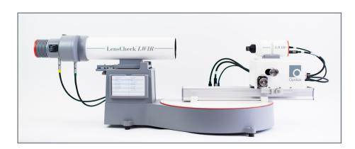
Loosen the rail clamps without calibration decals with an M4 hex wrench.
