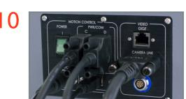
Plug in the power cable and computer cables as shown.
