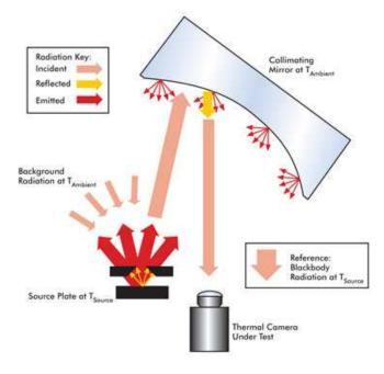
The cooler background radiation does not compensate entirely for the imperfect emissivity of the target, and the radiation from the ambient temperature mirror does not fully compensate for its imperfect reflectivity. The result is that the radiation presented to the camera under test appears to have originated from a blackbody at a temperature less than the physical temperature of the source.
