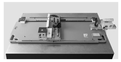
The Finite Conjugate Lens Measurement Instrument is available as a *standalone* unit or as a LensCheck™ VIS *option*. When used as a LensCheck option for measuring finite distances, the LensCheck™ Image Analyzer (IA), IA Mount and Lens Mount are removed from the LensCheck unit and mounted to the instrument base. The image may then be moved to a precise location on the rail, and may be moved off axis.
