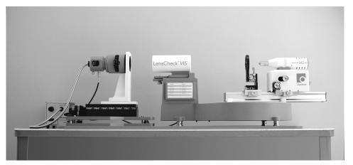
The Adjustable Conjugate Lens Instrument is available as a standalone unit or by customizing your LensCheck. It allows you to measure lenses at any object distance—from -1m to infinity to +1.2m for real object distances; and at any field angle within +/- 110°. The negative conjugates are used for applications such as virtual reality, where the image is formed behind the lens you are testing.
