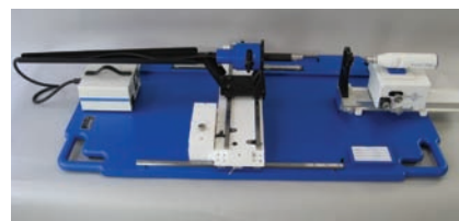
Figure 4. A tabletop bench allows for finite conjugate testing.
