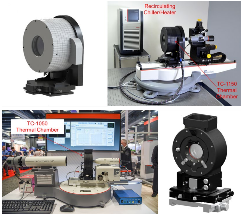
Figure 3 The TM-1150 thermal chamber (top left) is intended for large lens assemblies and can be mounted on an OpTest ® bench rotary platform as shown in the top right. The TM-1050 thermal chamber (bottom right) is intended for smaller lens assemblies that would typically be tested on a LensCheck ™ VIS test bench (bottom left)
