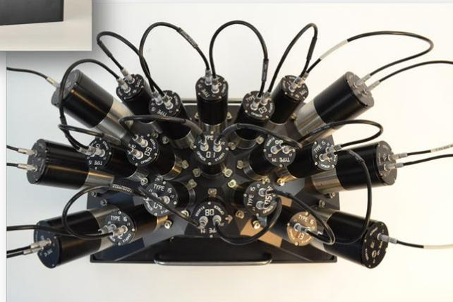
The Meridian Starfield mount consists of a thick plate into which precision bores are machined to receive the target projector barrels. This allows for consistent and repeatable testing of field points. When provided with a customer's camera lens prescription or black box model, Optikos can design unique targets to compensate for high distortion field points for ultra wide FOV cameras.
